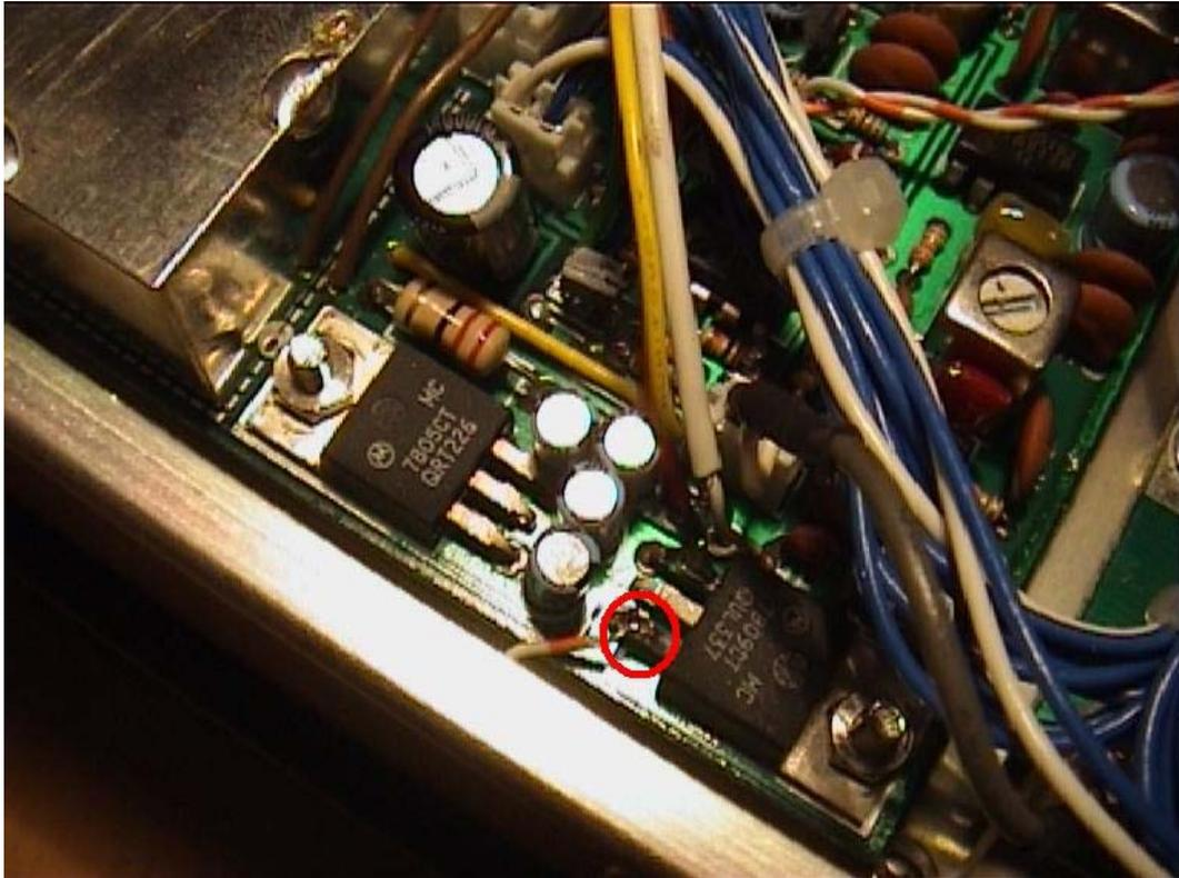
**Figure 3: IF/AF board showing 9v power take-off point for mixer**
