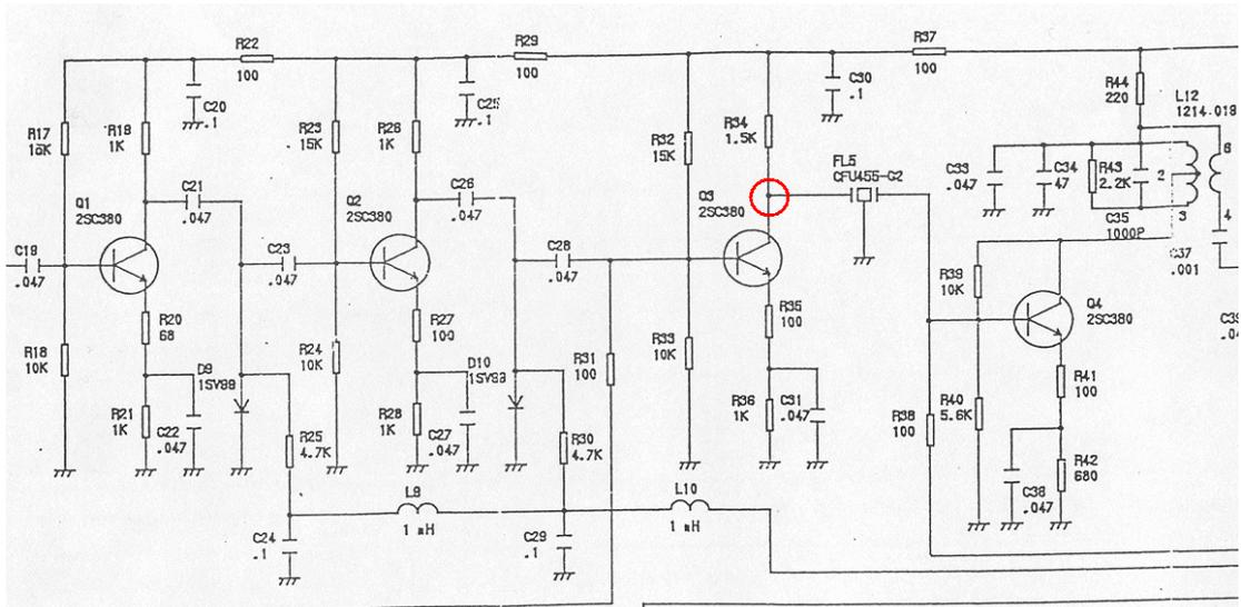
**Figure 1: Circuit of IF/AF board (part) showing take-off point for mixer**
