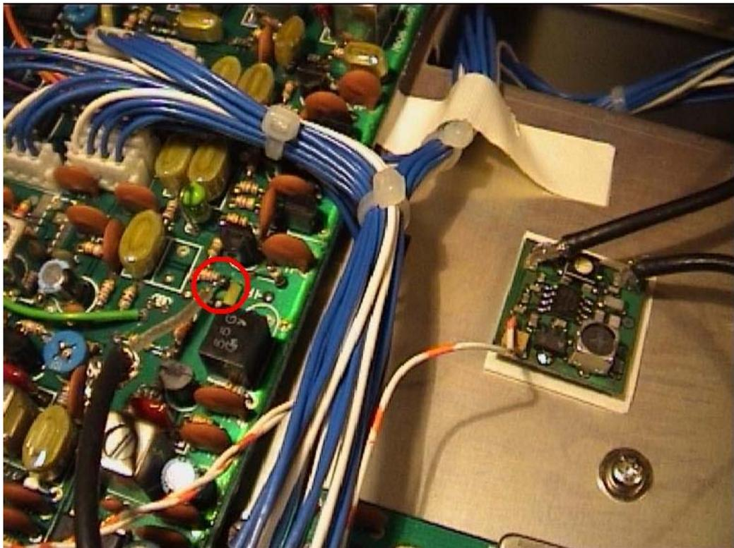
**Figure 2: IF/AF board, showing take-off point for mixer**
