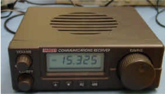
**Summary.** The receiver was modified and capable of receiving DRM, but performance was limited by the phase noise from the 1<sup>st</sup> Local Oscillator (LO).
